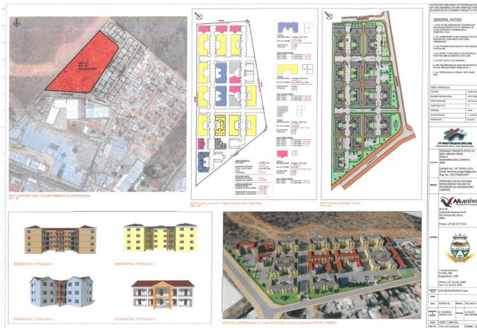
Figure 2. 12: Site development Plan for the proposed social housing on erf 479 Burgersfort extension 10.
